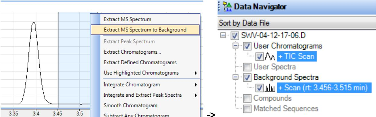
The screenshot shows a chromatogram with a peak highlighted. A context menu is open over the peak, listing several actions. The 'Extract MS Spectrum to Background' option is highlighted. To the right, the 'Data Navigator' window is visible, showing a tree view of data files. The file 'SwW-04-12-17-06.D' is expanded, showing 'User Chromatograms' with a '+ TIC Scan' button, 'User Spectra', 'Background Spectra' with a '+ Scan (rt: 3.456-3.515 min)' button, 'Compounds', and 'Matched Sequences'.
